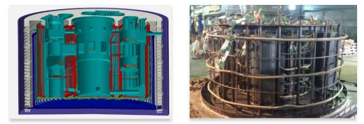
Figure LFR3. Reactor vessel computational model and mock-up
