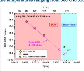
Figure SCWR 9. Comparison of the SCC and creep CGRs of Alloy 690 in subcritical and supercritical water at the temperatures ranging from 360°C to 550°C
