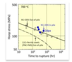
Figure SFR 7. Comparison of In-pile and Out-of-pile creep rupture strength of 9Cr-ODS TMS
