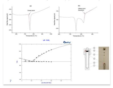
Figure MSR 4. Phase diagram study pf the LiF-PuF3 system
