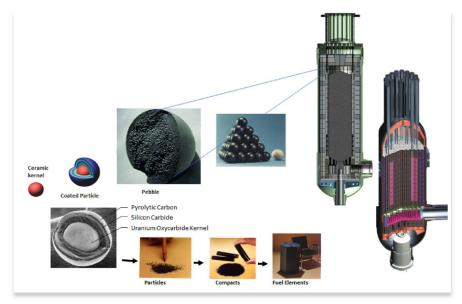
Figure VHTR 1. TRISO coated-particle fuel as the basis for hexagonal block and pebble bed core designs
