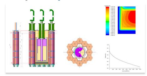
Figure MSR 5. Design of the heated zone for FLIBE salt
