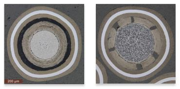
The US AGR-5/6/7 irradiation of UCO TRISO fuel continues in the Advanced Test Reactor. This experiment is both the final fuel qualification irradiation and a separate high-temperature fuel performance margin test (peak temperatures of ~1 500°C) and contains approximately 570 000 fuel particles in 194 fuel compacts. The irradiation is roughly half complete.
