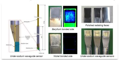
Figure SFR 8. Waveguide sensors fabricated for sodium-wetting tests
