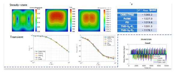
Figure MSR 3. Multi-physics code for V&V. Benchmark of PoliMi and PSI codes
