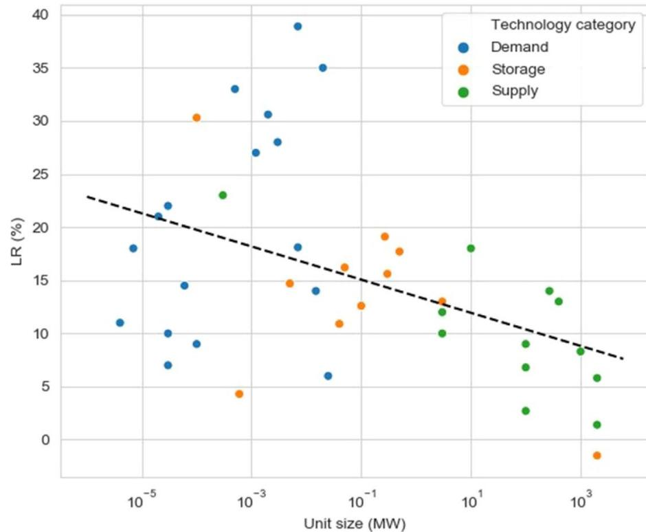
**Figure 1. LRs for 41 Energy Technologies**
