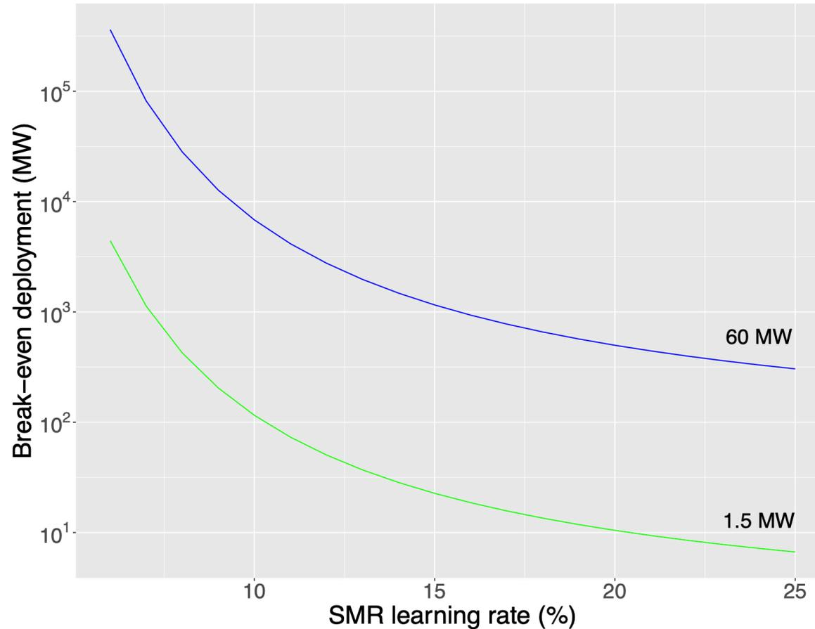
SMR deployment needed to reach cost-parity with an AP1000 reactor, assuming it starts at \$5,500/kW, 1,100MW and a learning rate of 1%. The break-even deployment is shown as a function of learning rate for the 60MW reactor (in blue) and the 1.5MW reactor (in green), assuming both start at \$11,000/kW.
