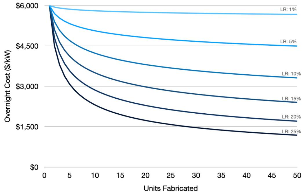
Learning curves for a generic SMR as a function of units fabricated and learning rate. The starting cost for every curve is \$6,000/kW.
