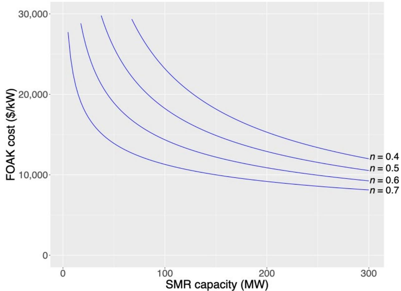
Illustration of the standard scaling relation for a base plant of  $OCC = \$5,500/kW$  and  $Capacity = 1100MW$ . The blue lines show the first-of-a-kind cost for an SMR as a function of size in MW for four different scaling factors. (For an example of how these factors are applied, see IAEA (2013))
