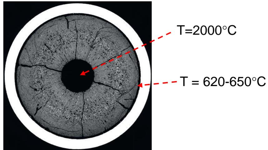
Transversal macrograph of a fuel pin after irradiation in a SFR (2)
