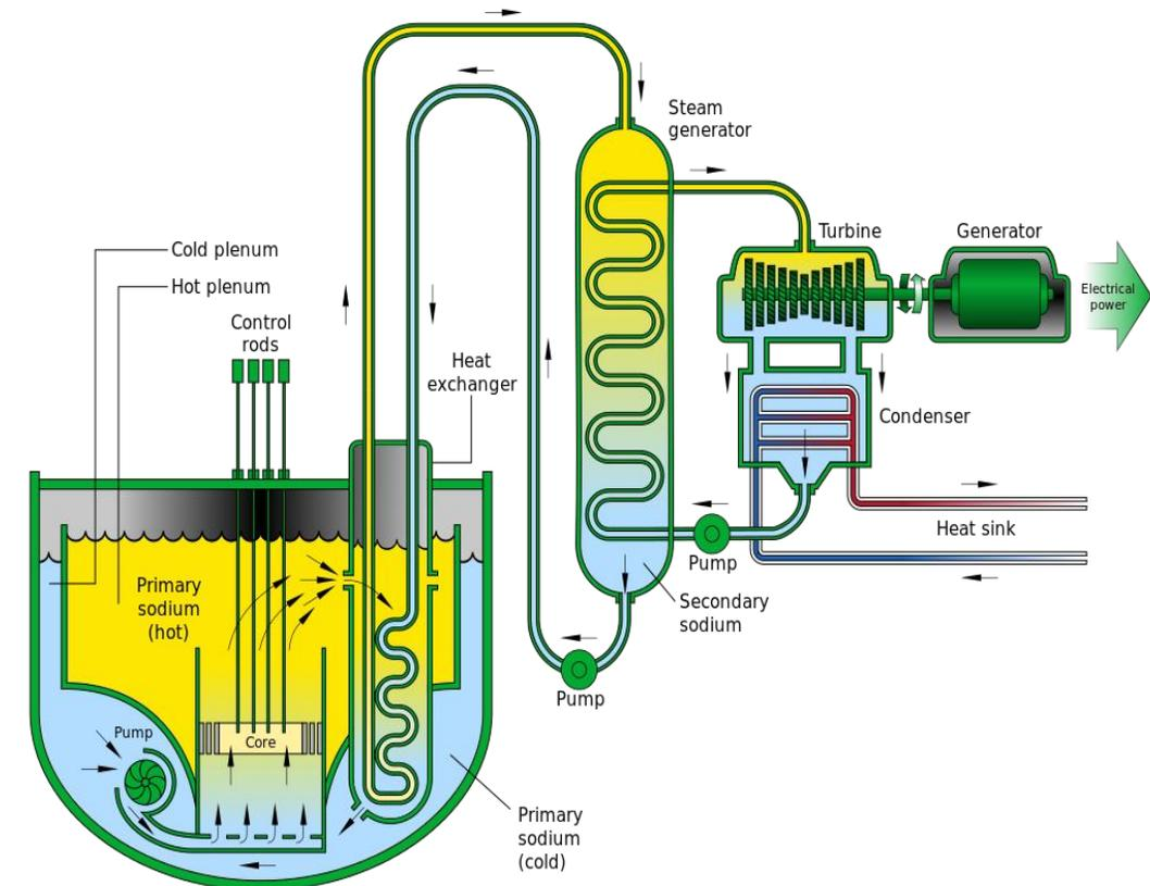
Sketch of a Sodium-cooled Fast Reactor (1)
