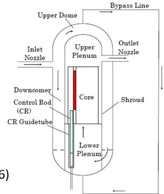
Japan's Pressure-Vessel Type SCWR Core Concept (Yamada et al., 2011)
