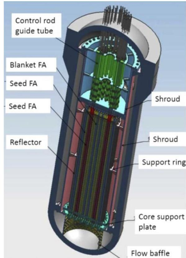
Japan's Fast-Spectrum SCWR Core Concept (Schulenberg et al., 2014)
