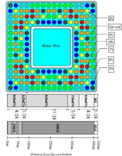
Japan's Pressure-Vessel Type SCWR Fuel Concept (Sakurai et al., 2011)
