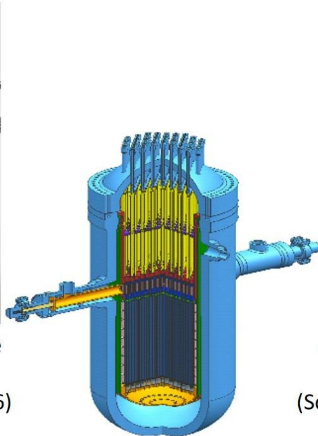
China's Pressure-Vessel Type SCWR Core Concept (IAEA, 2015)
