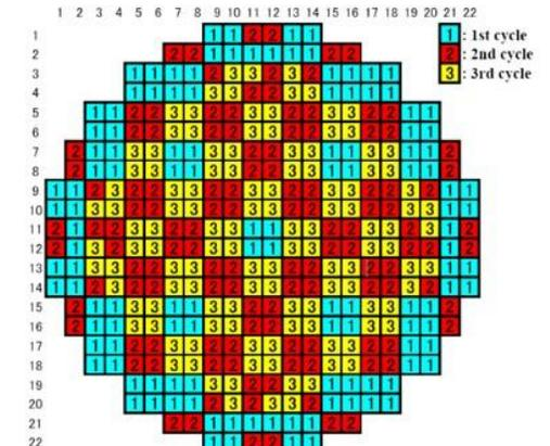
Japan's Thermal Spectrum SCWR Core Map (Yamada et al., 2011)
