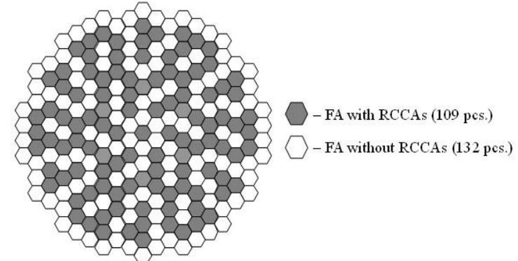
Russian Federation's Fast Spectrum SCWR Core Map (Ryzhov et al., 2011)
