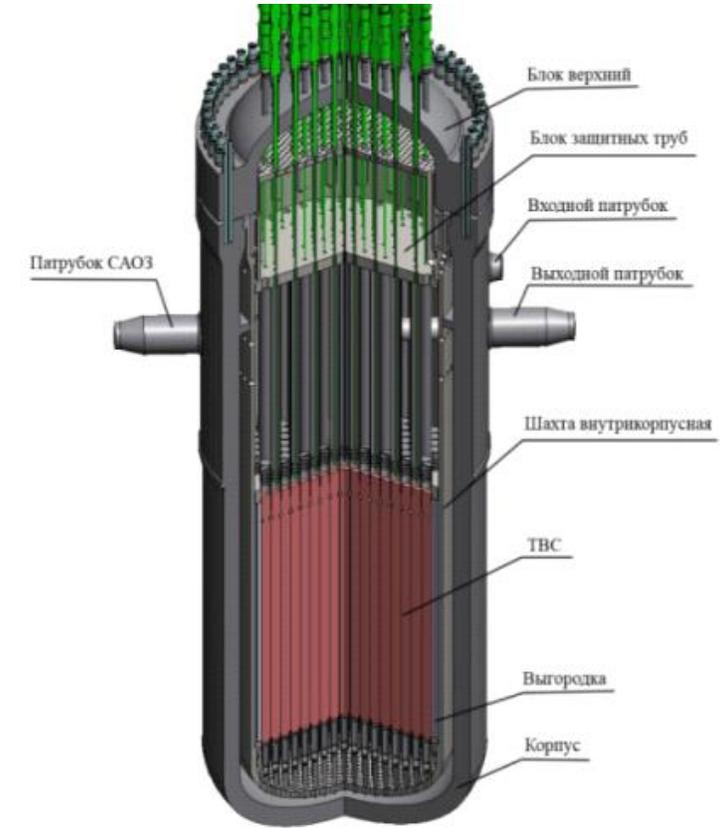
Russian Federation's Fast Spectrum SCWR Core Concept (Ryzhov et al., 2011)
