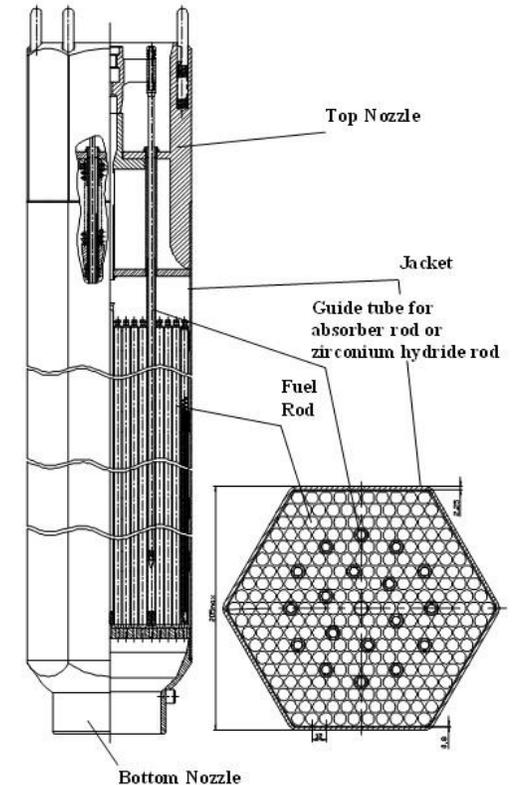
Russian Federation's Fast Spectrum SCWR Fuel Concept (Ryzhov et al., 2011)
