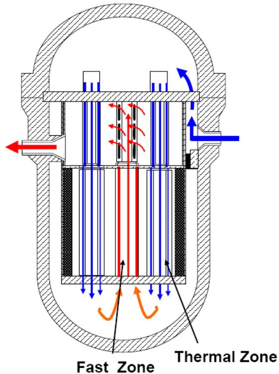
China's Mixed-Spectrum SCWR Core Concept (Cheng et al., 2007)
